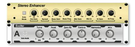
**ENHANCERS** let you emphasize the Bass, Midrange and Hi output at selectable frequencies, allowing you to generate maximum punch, clarity and detail – without turning up the overall volume. (Inspired by SPL Vitalizer\*)
